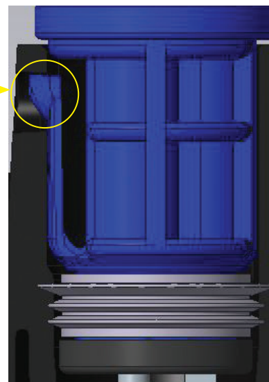
Modulator Valve Solenoid Cut-Away Section Showing Tab In Locked Position
